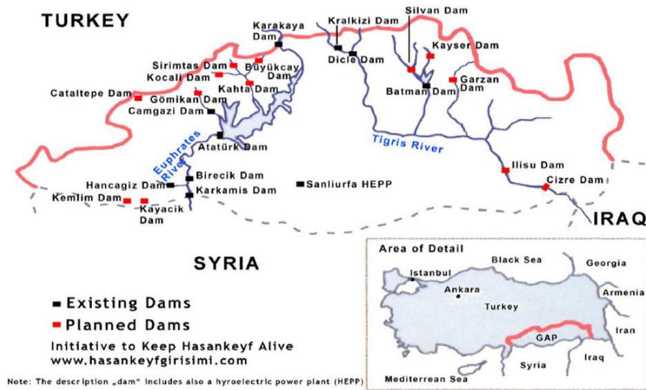
Figure 3: Locations of Built and Under-Construction Dams on the Tigris and Euphrates Rivers in the Southeastern Anatolia Project (GAP) in Turkish Territory (Salameh & Al-Ansari, 2021)
